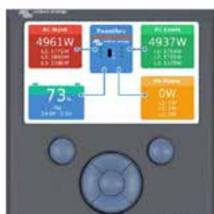
Color Control GX, showing a PV application
