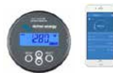
BMV-712 Smart Battery Monitor The BMV Battery Monitor features an advanced microprocessor control system combined with high resolution measuring systems for battery voltage and charge/discharge current. Besides this, the software includes complex calculation algorithms, like Peukert's formula, to exactly determine the state of charge of the battery. The BMV selectively displays battery voltage, current, consumed Ah or time to go. The monitor also stores a host of data regarding performance and use of the battery.
